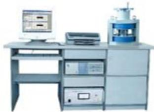
Automatic measurement on hysteresis loop and demagnetization curve of permanent-magnet material, accurate measurement on magnetic characteristic parameters such as remanence Br, coercive force HcB, intrinsic coercive force HcJ and maximum magnetic energy product (BH)max.
