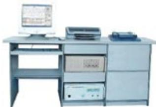
Automatic measurement on dynamic hysteresis loop of soft magnetic (silicon steel) material under 50Hz, 60Hz, 400Hz and 1kHz, accurate measurement on dynamic magnetic characteristic parameters such as amplitude permeability  $\mu_a$ , loss angle  $\delta$ , total losses  $P_s$ , remanence  $B_r$  and coercive force  $H_c$ .
