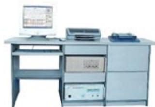
Automatic measurement on dynamic hysteresis loop of soft magnetic (silicon steel) material under 50Hz, 60Hz, 400Hz and 1kHz, accurate measurement on dynamic magnetic characteristic parameters such as amplitude permeability  $\mu_a$ , loss angle  $\delta$ , total losses  $P_s$ , remanence  $B_r$  and coercive force  $H_c$ .
