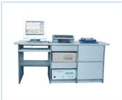
Automatic measurement on dynamic hysteresis loop of soft magnetic (silicon steel) material under 50Hz, 60Hz, 400Hz and 1kHz, accurate measurement on dynamic magnetic characteristic parameters such as amplitude permeability  $\mu_a$ , loss angle  $\delta$ , total losses  $P_s$ , remanence  $B_r$  and coercive force  $H_c$ .
