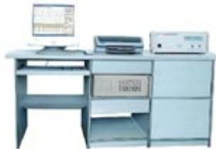
Automatic measurement on hysteresis loop of soft magnetic material under dynamic (AC) condition, accurate measurement on dynamic magnetic characteristic parameters such as amplitude permeability  $\mu_a$ , loss angle  $\delta$ , iron loss  $P_c$ , remanence  $B_r$  and coercive force  $H_c$ .
