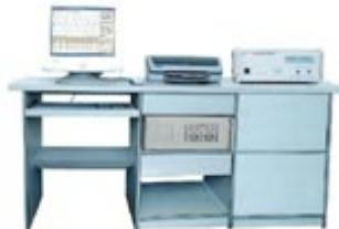
Automatic measurement on hysteresis loop of soft magnetic material under dynamic (AC) condition, accurate measurement on dynamic magnetic characteristic parameters such as amplitude permeability  $\mu_a$ , loss angle  $\delta$ , iron loss  $P_c$ , remanence  $B_r$  and coercive force  $H_c$ .
